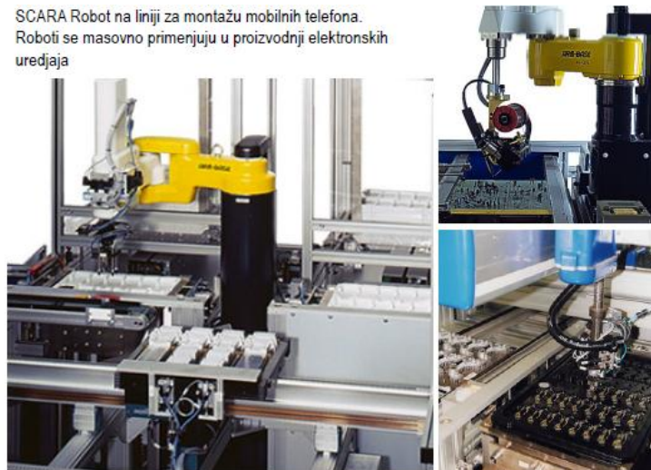
Picture 2. Robotic assembling - a robot at the cell phones assembly line
